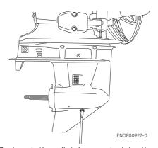
Insert the oil tube nozzle into the lower oil plug hole, and fill with gear oil by squeezing the oil tube until oil flows out of the upper plug hole and bubbles is disappeared to remove the air.
