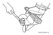
5. Install a new split pin into the nut hole and bend it.
