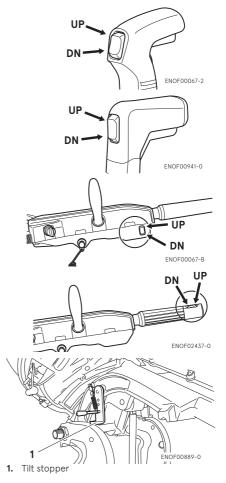
The outboard motor can also be tilted up and down using the switch provided on the bottom cowl.
