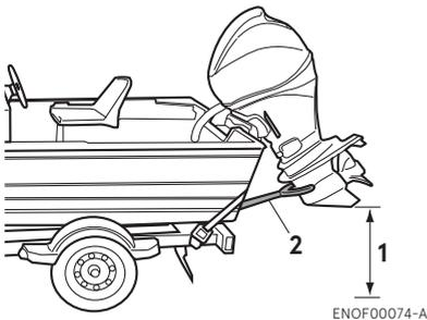
1. Ground clearance should be provided sufficiently.
