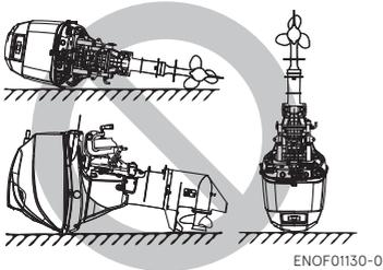
Keep the outboard motor in a vertical position when carrying. The optional outboard motor stand is recommended for keeping the outboard motor vertical both during transport and storage.
