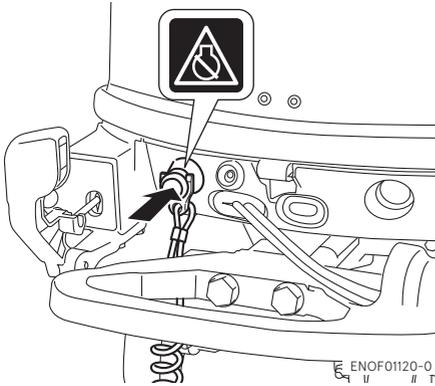
4. Turn the main switch key to the OFF position or push the stop switch. ( Do not forget to turn the key off).
