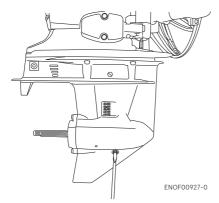
Insert the oil tube nozzle into the lower oil plug hole, and fill with gear oil by squeezing the oil tube until oil flows out of the upper plug hole and bubbles is disappeared to remove the air.
